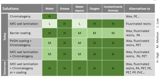
MFC : Micro Fibrillated cellulose Chromatogeny<sup>TM</sup> : Brings hydrophobicity to hydrophilic reactive substrates.
